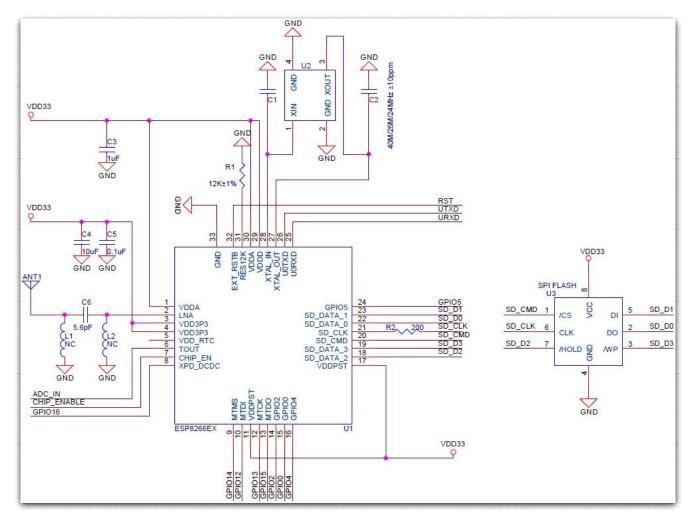
Figure 4 Schematics of ESP-12F WiFi Module
